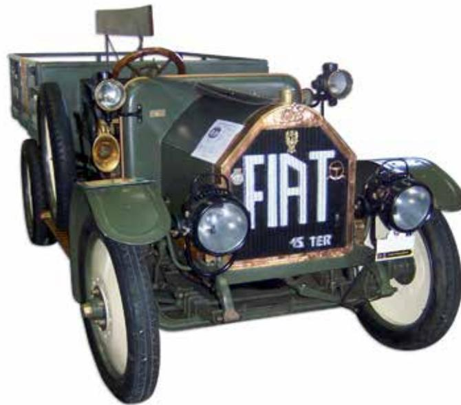
In 1909, by order of the army of the King of Italy, Fiat studied a new multifunctional truck for transporting troops and materials, and presented the famous Fiat 15, installing for the first time on this type of vehicle a petrol pump to replace the gravity feed design. The 15 model was a roaring success and further versions were then produced the 15 Bis, named Libia, and the 15 Ter equipped with a more powerful engine.
