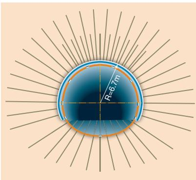
Left: Fig 6 - Profile 2 lining, with Phase 1 marked in blue and Phase 2 in orange
